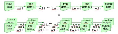
With a multi-cores PC or a computational cluster (ex. 2000 cores), we can attribute one core to one workflow.
